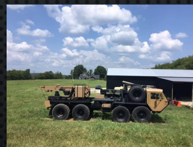
Hybrid between M983 HEMTT and M936 wrecker
